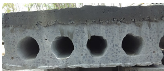
(b) Hollow Core Slabs with Bonded Overlay
