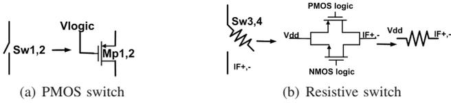
Fig. 5. Switch implementation using MOS
