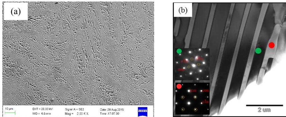
**Figure 1.** (a) SEM and (b) TEM micrographs of the as-cast EHEA showing the lamellar microstructure. The inset SADPs (marked by green and red spots) obtained from green and red spots in (b) correspond to the  $L1_2$  with zone axis  $[011]$  and B2 phase with zone axis  $[001]$ , respectively.
