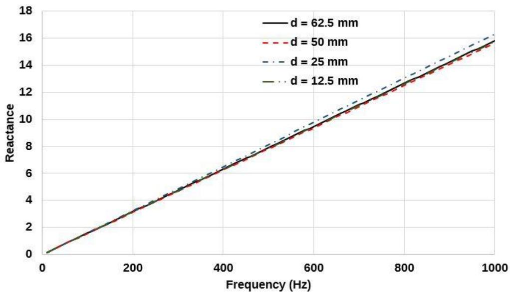
Figure 8: Variation of reactance with inner tube diameter (d) in CTR configuration
