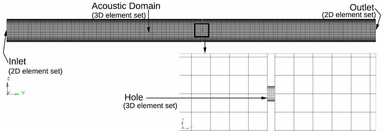
Figure 4: Meshed model of impedance tube with single hole sample
