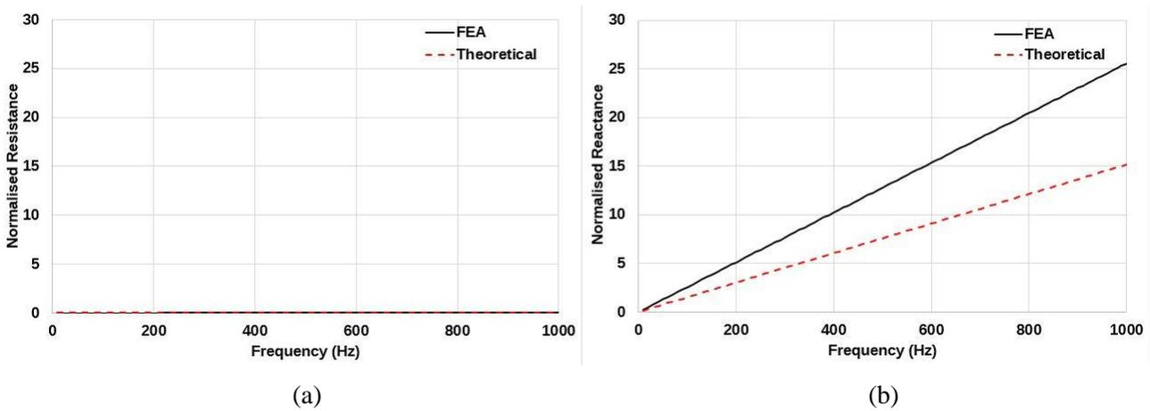
Figure 6: Comparison between FEA and theoretical results (a) normalized resistance (b) normalised reactance
