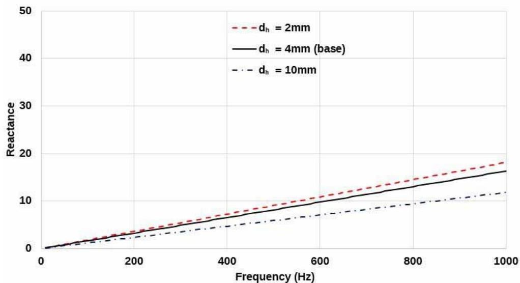
Figure 10: Variation of reactance with hole diameter ( $d_h$ )
