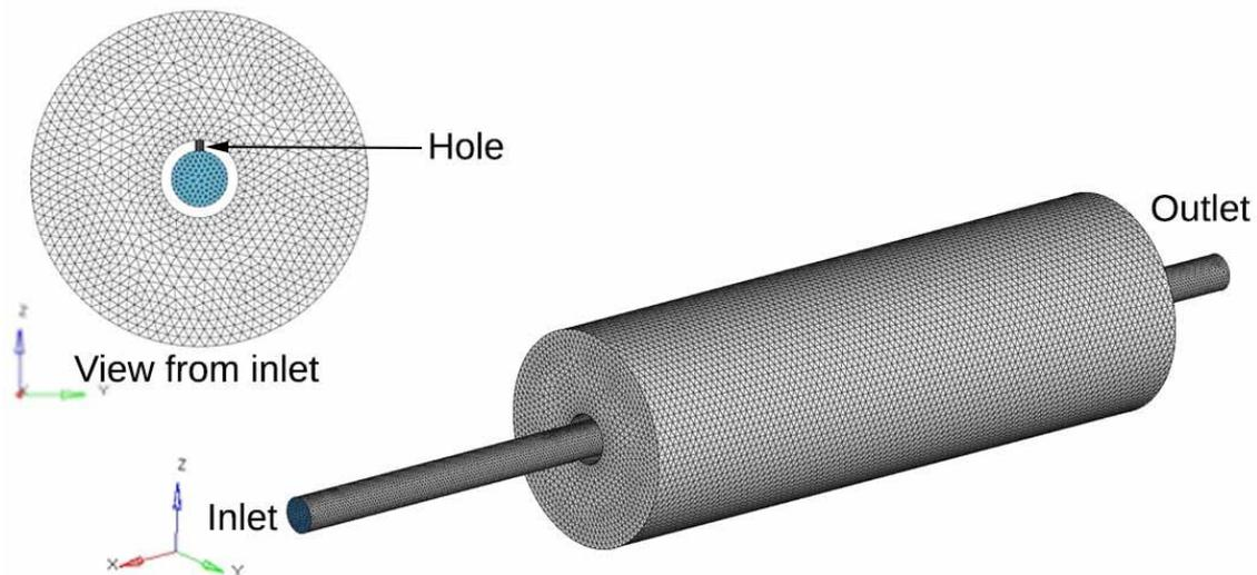
Figure 5: Meshed model of CTR with single hole
