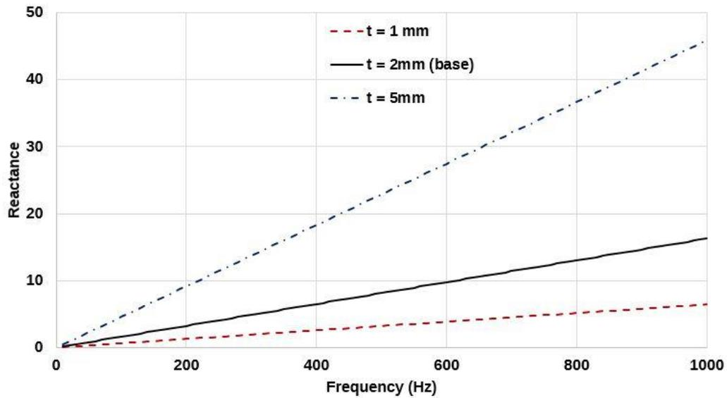
Figure 9: Variation of reactance with liner wall thickness ( $t$ )
