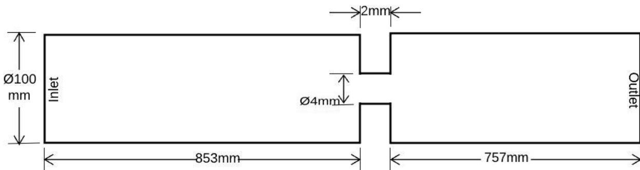
Figure 1: Computational domain of impedance tube with single hole sample
