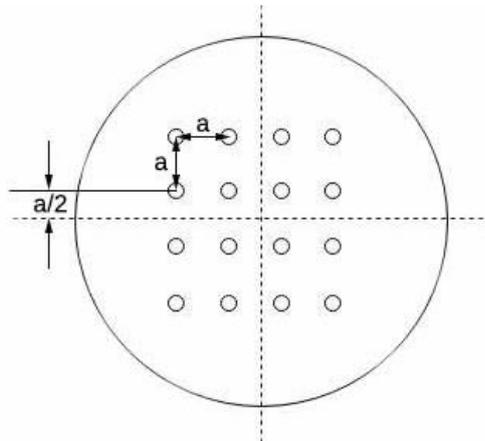
Figure 2: Multiple hole sample configuration with 16 holes with spacing 'a'
