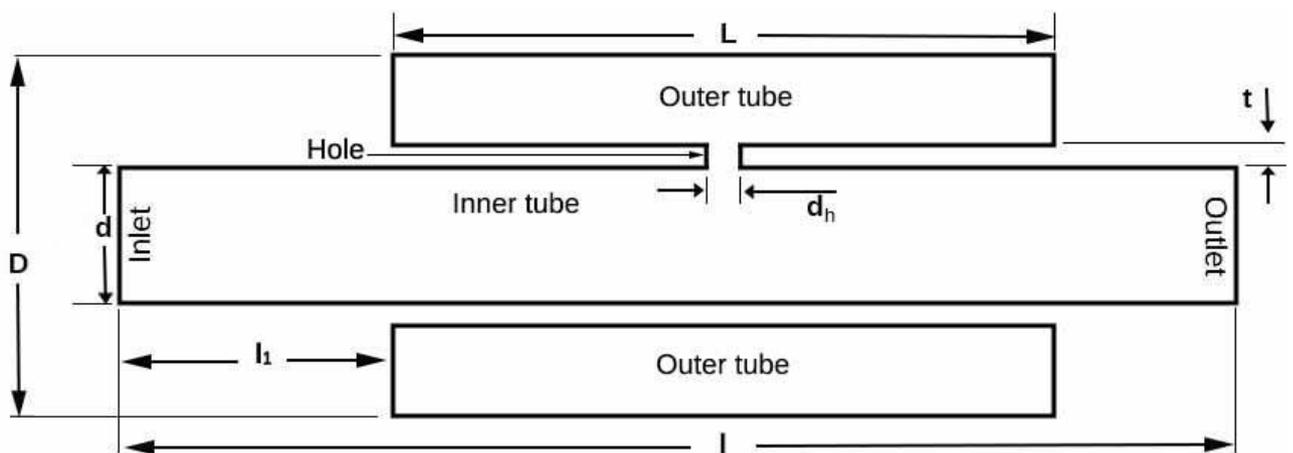
Figure 3: Computational domain of CTR with single hole
