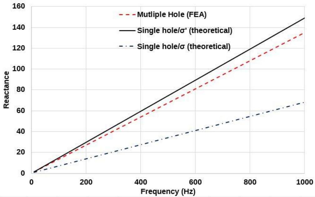
Figure 7: Comparison of reactance of multiple hole FEA model and theoretical model
