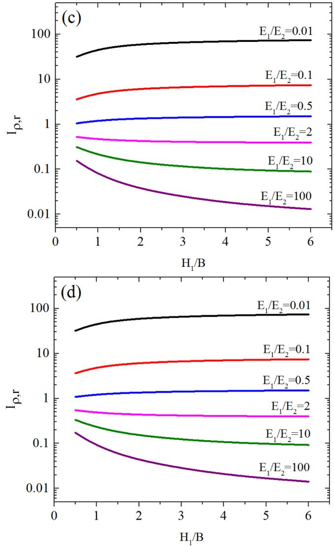
**Fig. 5** Settlement influence factor for rigid footing for  $L/B=1$  for various  $H_1/B$  and  $E_1/E_2$  values corresponding to (a)  $H_2/B=1$ , (b)  $H_2/B=2$ , (c)  $H_2/B=4$ , and (d)  $H_2/B=6$
