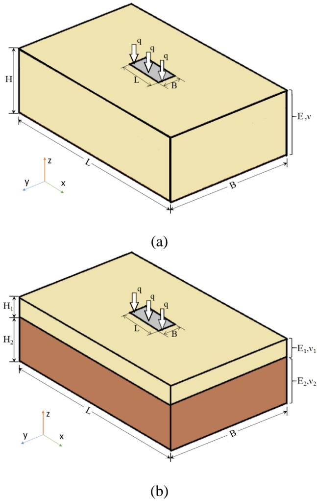
**Fig. 1** Schematic showing a rigid footing resting on a) finite layer of soil, and b) two-layered soil system underlain by a rigid base
