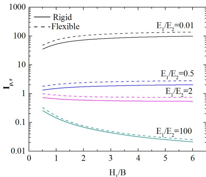
**Fig. 8** Variation of settlement factors with  $H_1/B$  values for rigid and flexible footings for  $L/B=2$ , and  $H_2/B=4$
