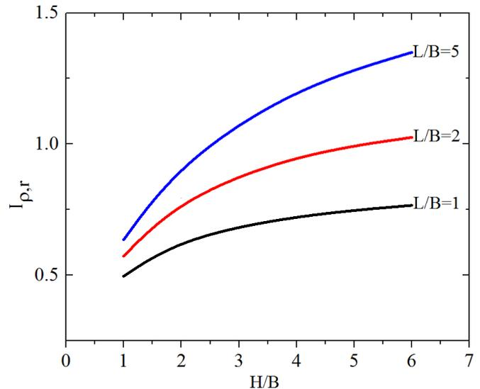
**Fig. 4** Settlement influence factor for rigid footings resting on finite layer of soil
