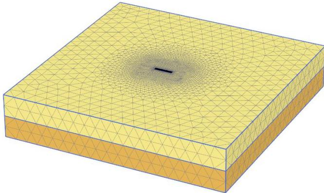
**Fig. 2** Finite element model in PLAXIS 3D v 2013 for the case of  $L/B=5$ ,  $H_1/B=6$ ,  $H_2/B=6$ ,  $E_1/E_2=100$  for a two-layered soil system
