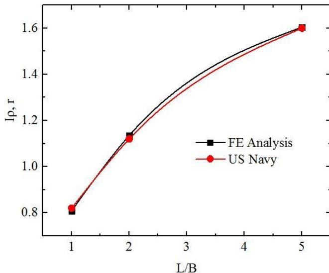
**Fig. 3** Comparison of settlement influence factors from FE model and US Navy manual for the case of footing resting on a semi-infinite layer of soil
