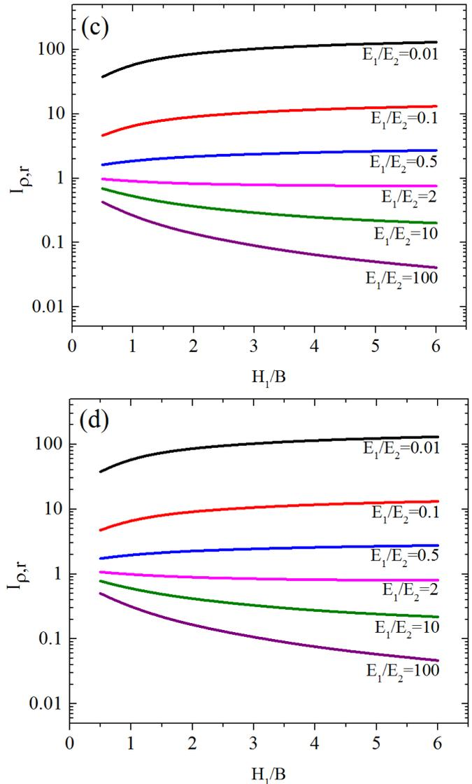
**Fig. 7** Settlement influence factor for rigid footing for  $L/B=5$  for various  $H_1/B$  and  $E_1/E_2$  values corresponding to (a)  $H_2/B=1$ , (b)  $H_2/B=2$ , (c)  $H_2/B=4$  and (d)  $H_2/B=6$
