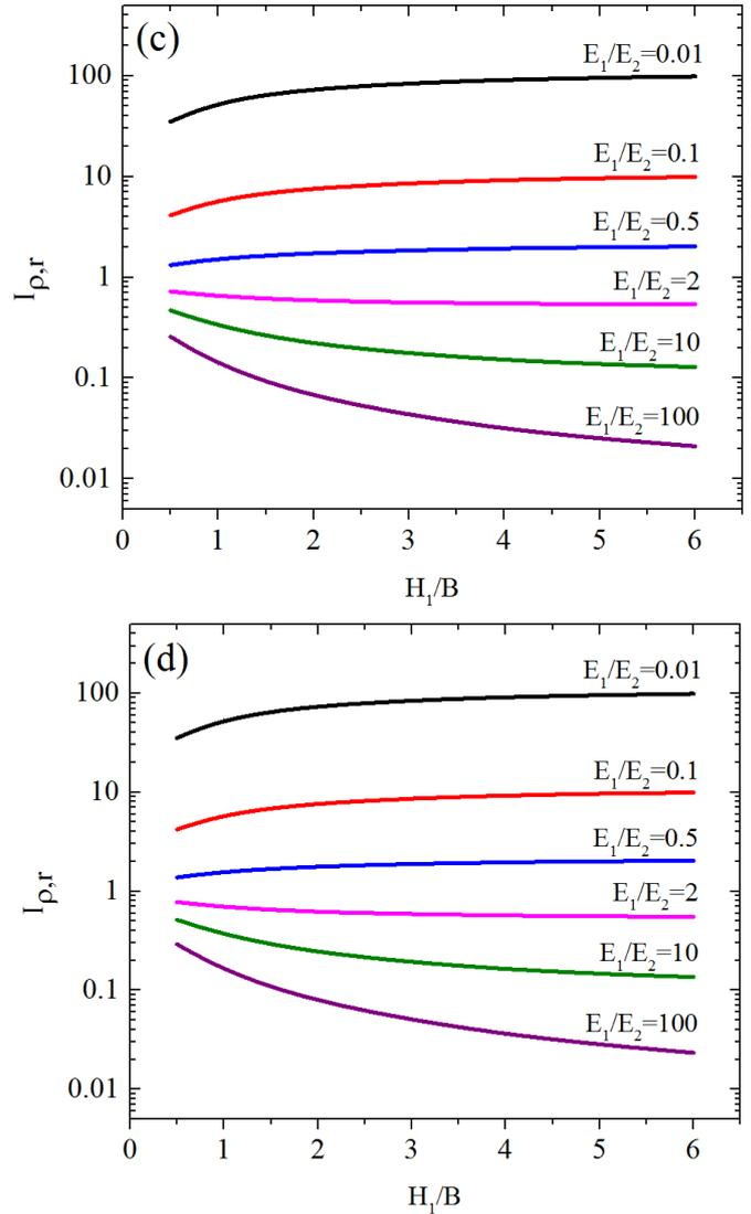
**Fig. 6** Settlement influence factor of rigid footing for  $L/B=2$  for various  $H_1/B$  and  $E_1/E_2$  values corresponding to (a)  $H_2/B=1$ , (b)  $H_2/B=2$ , (c)  $H_2/B=4$  and (d)  $H_2/B=6$
