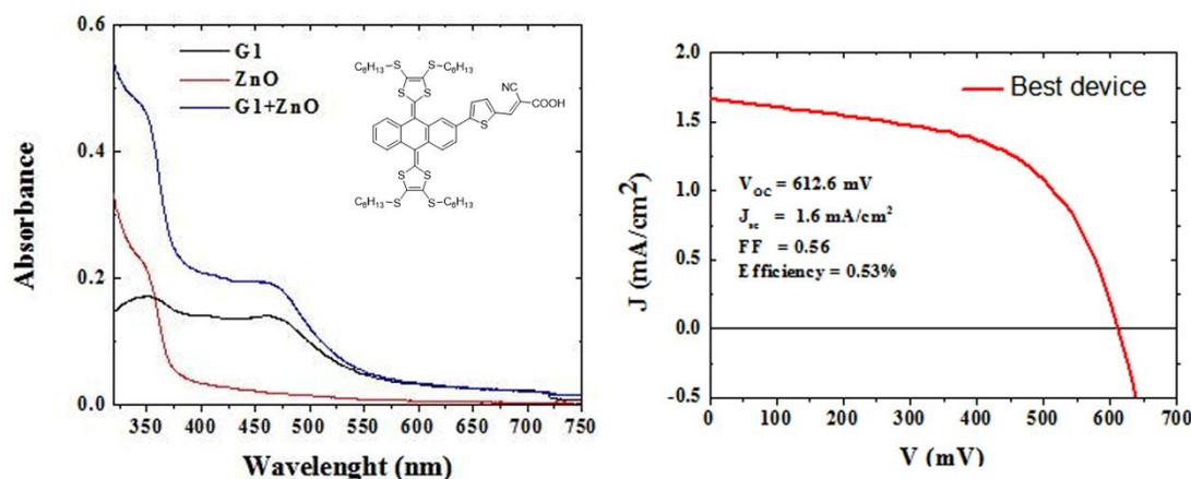
Fig. 1: (left) Absorption spectra of the G1 molecule and the G1+ZnO thin films on fused silica substrate; (right) photovoltaic device data of the fabricated DSSC
