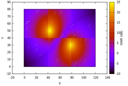
Fig. 7. Optimal Placement of Femtos in Floor 2
