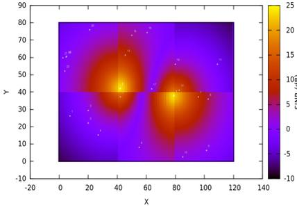
Fig. 8. Center Placement of Femtos in Floor 2
