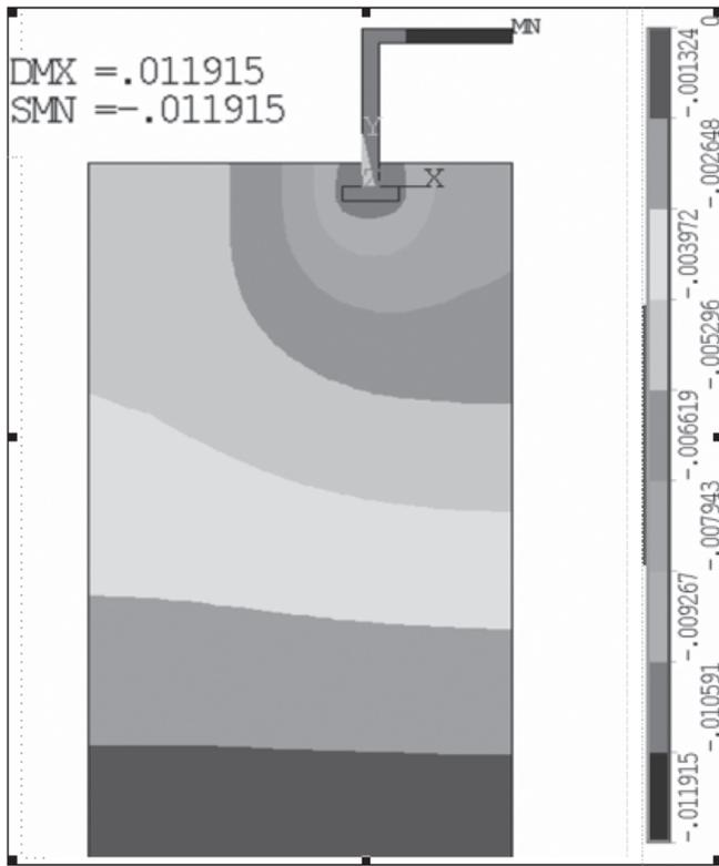
Fig. 9 Contour plot of displacement for Case 3
