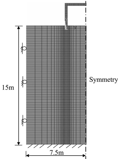
Fig. 6 Finite element meshing for Case 2 and Case 3
