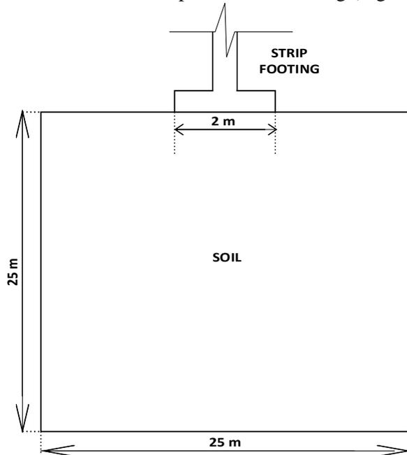
**Fig. 1** Schematic representation of soil and footing
