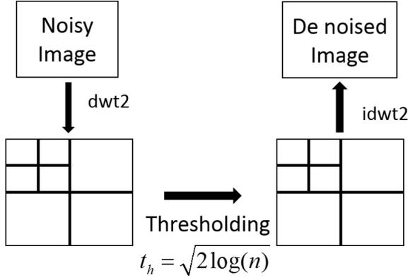
Fig. 4: Denoising using 2 level DWT: dwt2, idwt2
