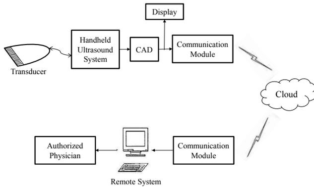
Fig. 1: Proposed cloud based ultrasound imaging system with CAD for preliminary diagnosis
