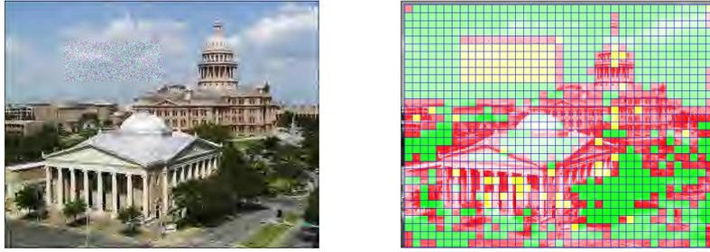
Fig. 7. JP2K Distorted Image from LIVE Database with added AWGN noise patch & its PIQUE Spatial Quality Mask. Where Red, Yellow and Green fill indicates blocks that satisfy NDC, NC and uniform criterions.
