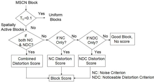
Fig. 2. Block level Distortion Classification and Quantification
