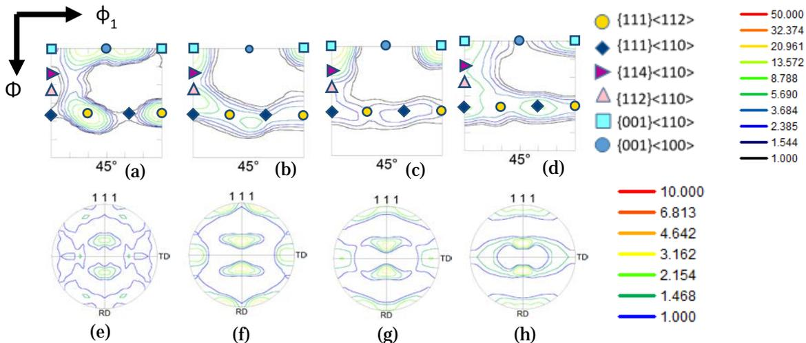
Fig. 1:  $\phi_2=45^\circ$  section of ODFs of ferrite in DSS (a) homogenized and warm-rolled at (b) 225°C, (c) 425°C and (d) 625°C. (111) PFs of austenite in DSS (e) homogenized and warm-rolled at (f) 225 °C, (g) 425°C and (h) 625°C.
