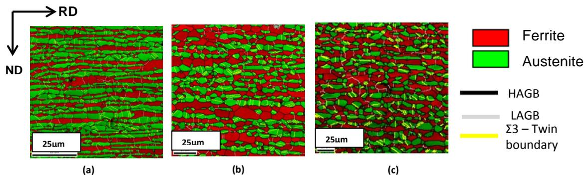
Fig. 2: Phase maps of DSS 90% warm-rolled at 625°C and annealed at 1175°C for (a) 2 minutes, (b) 30 minutes and (c) 120 minutes.
