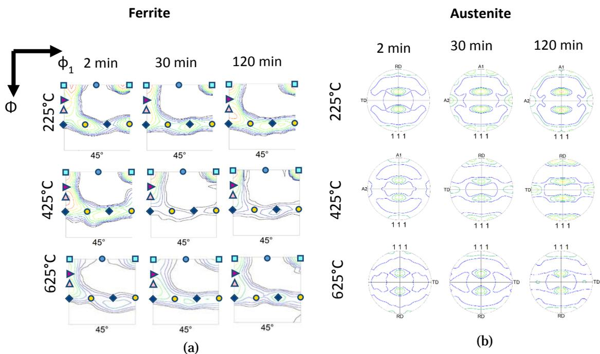
Fig. 3: (a)  $\phi_2=45^\circ$  section of ODFs of ferrite and (b) (111) PFs of austenite in DSS 90% warm-rolled at different temperatures and then isothermally annealed at 1175°C for different time intervals. The intensities of the contour lines are same as those shown in Fig.1.
