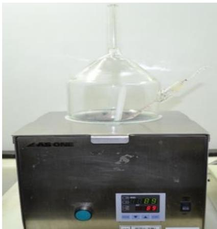
**Figure 2:** Constant temperature bath for anisotropic etching of silicon.
